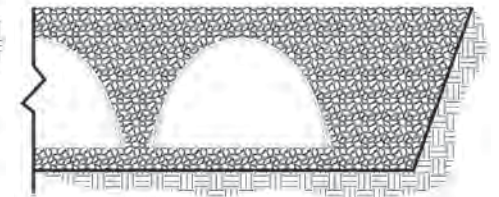
Perimeter Fully Backfilled
